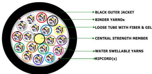
This cable is a stranded micro loose tube cable with optical fibre placed inside robust buffer tubes stranded around a fibre reinforced plastic (FRP) central strength member. In addition to optical fibres, the buffer tubes contain water blocking gel and the cable core is surrounded with water-absorbing yarns to prevent water from entering cable core.
